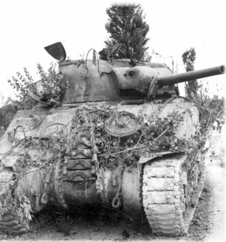
A photograph of Cpl. Thiessen's tank "Chilliwack II" the morning after she was holed twice by a 75mm. One round hit the Sherman's gun mantlet while a second round deflected off the bottom edge of the mantlet into the turret. Trooper Lavigne , the loader/operator, was the only casualty. The German Mk. IV tank was quickly knocked out by Lt. Hutching's crew in "Chicoutimi".
