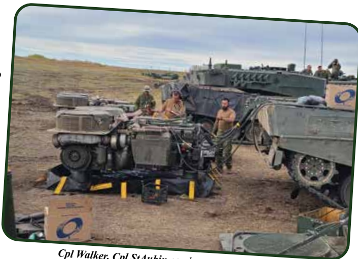
Cpl Walker, Cpl StAubin conduct a run-up checking for engine leaks alongside Sgt Crowe.
